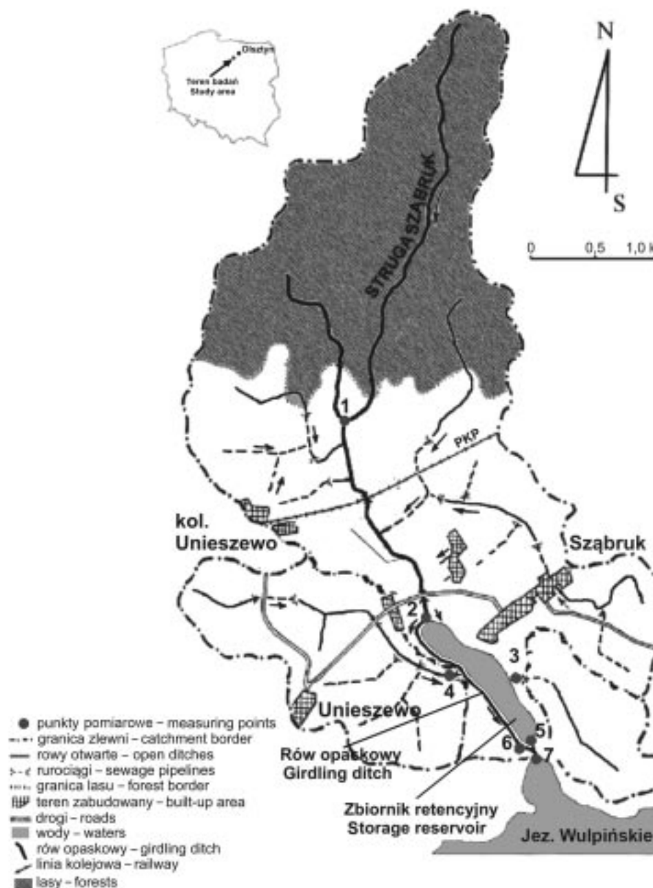
Fig. 1. Map of Sząbruk stream catchment area: 1 – Sząbruk stream below the afforested catchment, 2 – Sząbruk stream above the storage reservoir, 3 – inflow from the drained catchment to the storage reservoir, 4 – inflow from the drained catchment to the girdling ditch, 5 – outflow from the storage reservoir, 6 – outflow from the girdling ditch, 7 – inflow to Lake Wulpińskie
