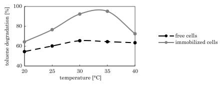
Fig. 4. Effect of temperature on degradation of free and immobilized cells
