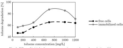
Fig. 5. Effect of initial toluene concentration on toluene degradation of free and immobilized cells
