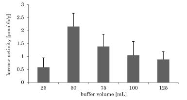
Fig. 1. Effect of buffer incubation volume on laccase activity in crude oil contaminated soil
