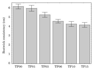
Fig. 3 Effect of mechanical treatment on Bostwick consistency of all tomato concentrate samples. Error bars represent standard deviation
