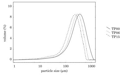
Fig. 1 Effect of mechanical treatment on the particle size distribution in tomato concentrate
