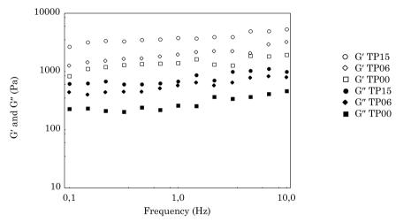
Fig. 4 Storage (G') and loss (G") moduli for samples TP00, TP06 and TP15 as a function of applied frequency
