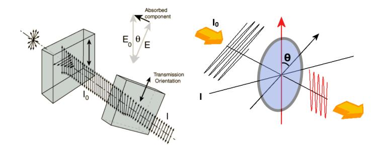
The polaroid material used in sunglasses makes use of dichroism, or selective absorption, to achieve polarization.
