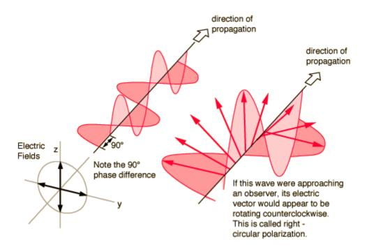
**Elliptical Polarization**. Elliptically polarized light consists of two perpendicular waves of unequal amplitude which differ in phase by 90°. The illustration shows right- elliptically polarized light.
