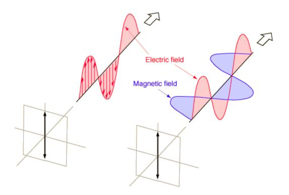
**Circular Polarization** Circularly polarized light consists of two perpendicular electromagnetic plane waves of equal amplitude and 90° difference in phase. The light illustrated is right-circularly polarized.
