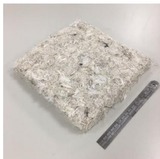
(a) Feather fibre fabric, density 29.8 kg/m 3
