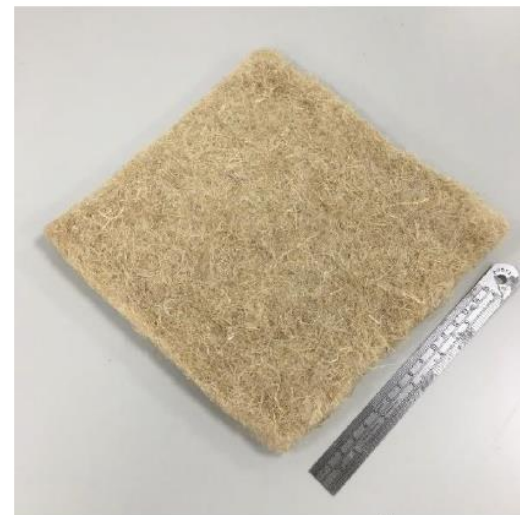
(c) Hemp fabric, density 83.3 kg/m 3
