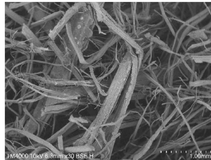
(f) Hemp fibre fabric SEM image
