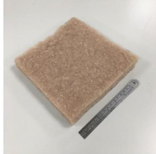
(g) PET fabric, density 25.5 kg/m 3
