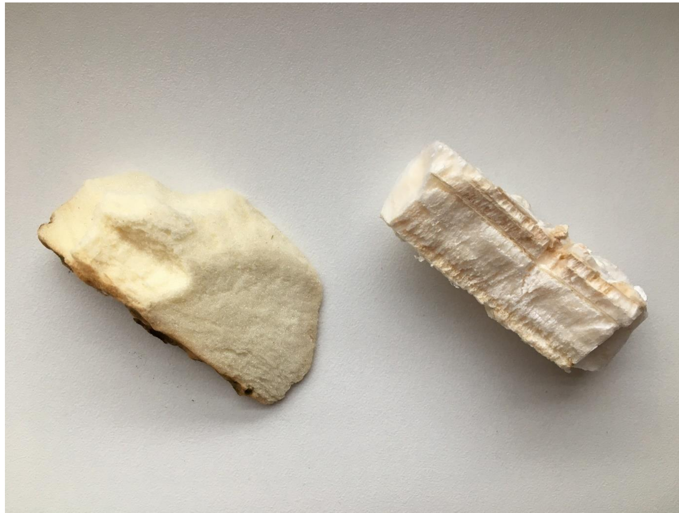
Samples of PIR thermal insulation and dried sunflower pith
