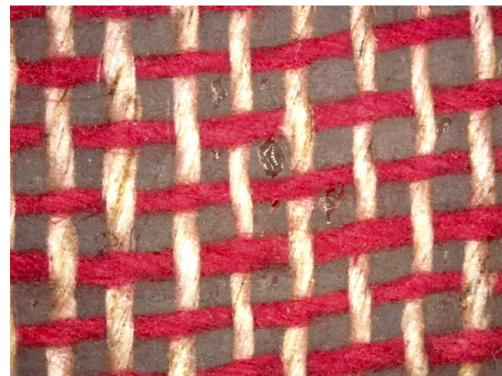
Imperfection in the matrix of sample
