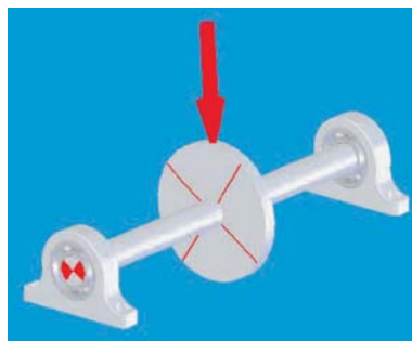
Fig. 1. The analyzed model of a rotor subjected to rotating transverse force
