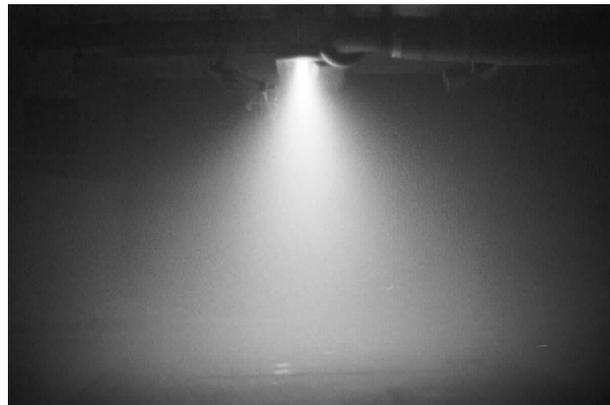
Fig. 1. The visible glow indicates that cold plasma is formed inside the process vessel, in which gas is irradiated.
