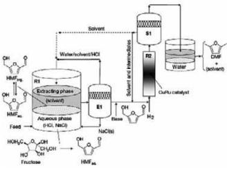
Fig. 7. The conversion of D-fructose into 2,5-DMF [11]
